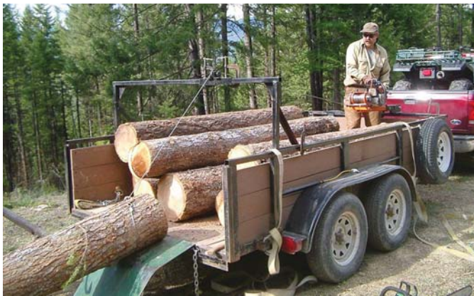
The Lewis Winch can be powered by any chainsaw motor that's 3 cu. in. or larger.
