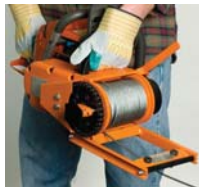
Winch is driven by a chainsaw with the bar and chain removed.
